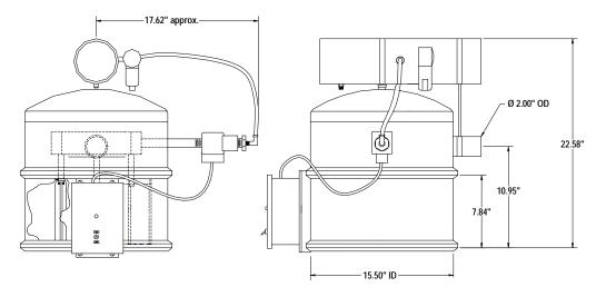
*Note:* The air inlet can be sized to vacuum system requirements using available transitions.
